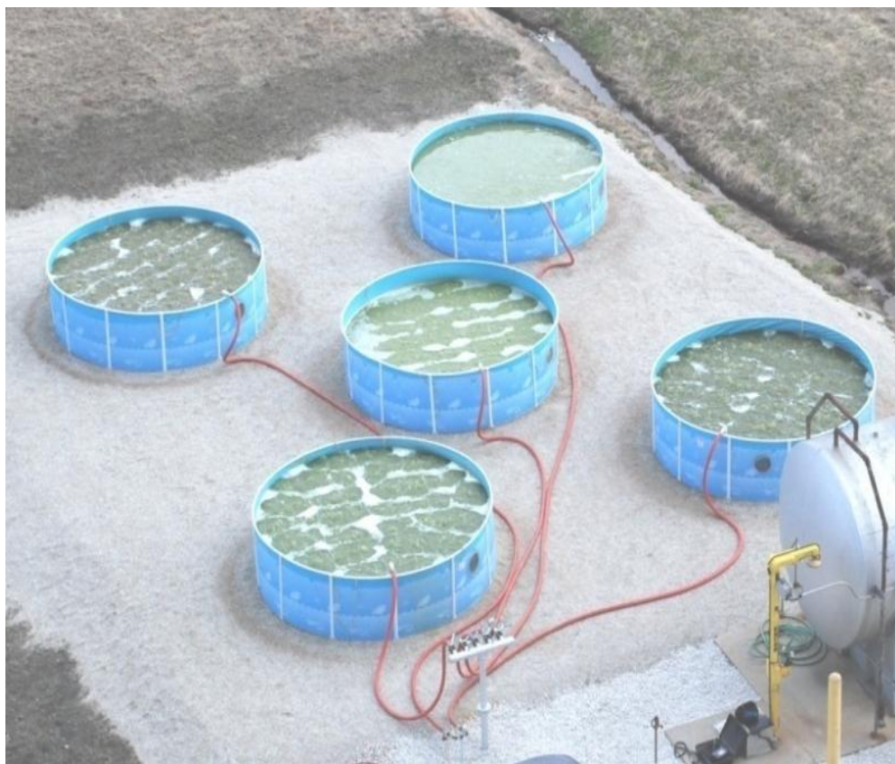
Figure 3.21. Flue gas from power plant captured by five 2500 gallon algae pools.
