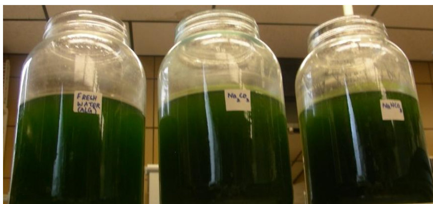
Figure 3.17. Scenedesmus algae grown with sodium carbonate (0.8 g/L) and sodium bicarbonate (0.63 g/L).
